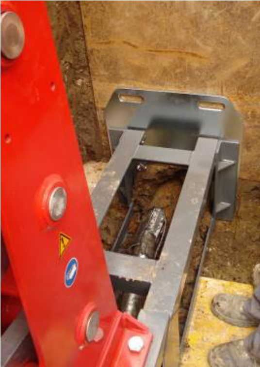
The roller cutter reaches the machine pit.
