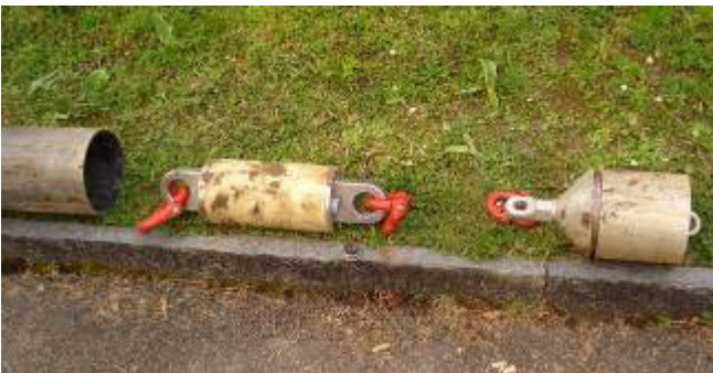
The measurement unit is assembled between the expander cone and the expander jack. The protection sleeve protects the measurement unit from damage through the broken fragments of the old pipe.
